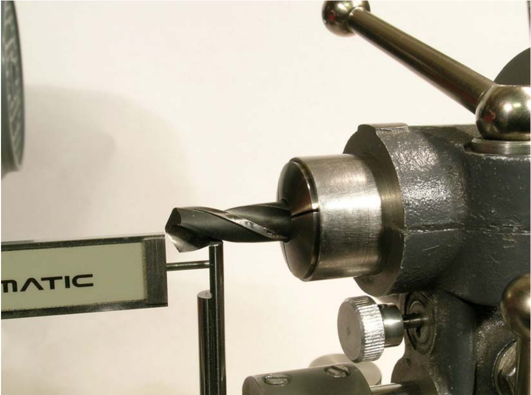
Figure 13: Setting drill tips distance R from the cone's axis
