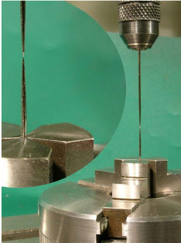
Figure 29: The table's zero position at the chucks centre.
