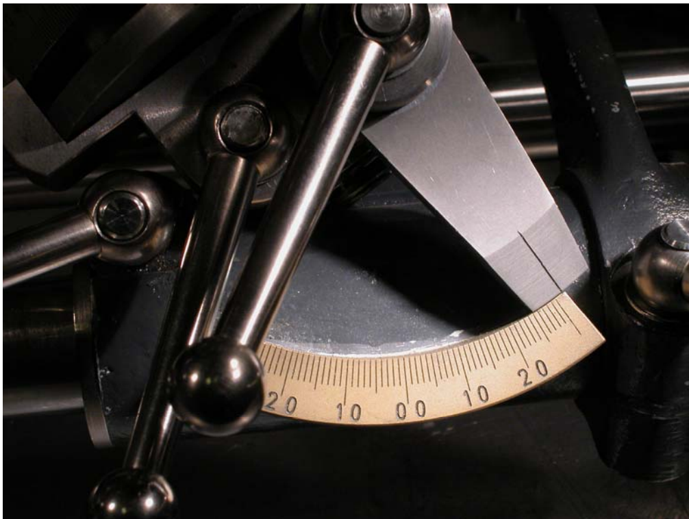
Figure 11: Setting the QUORN's tilting bracket
