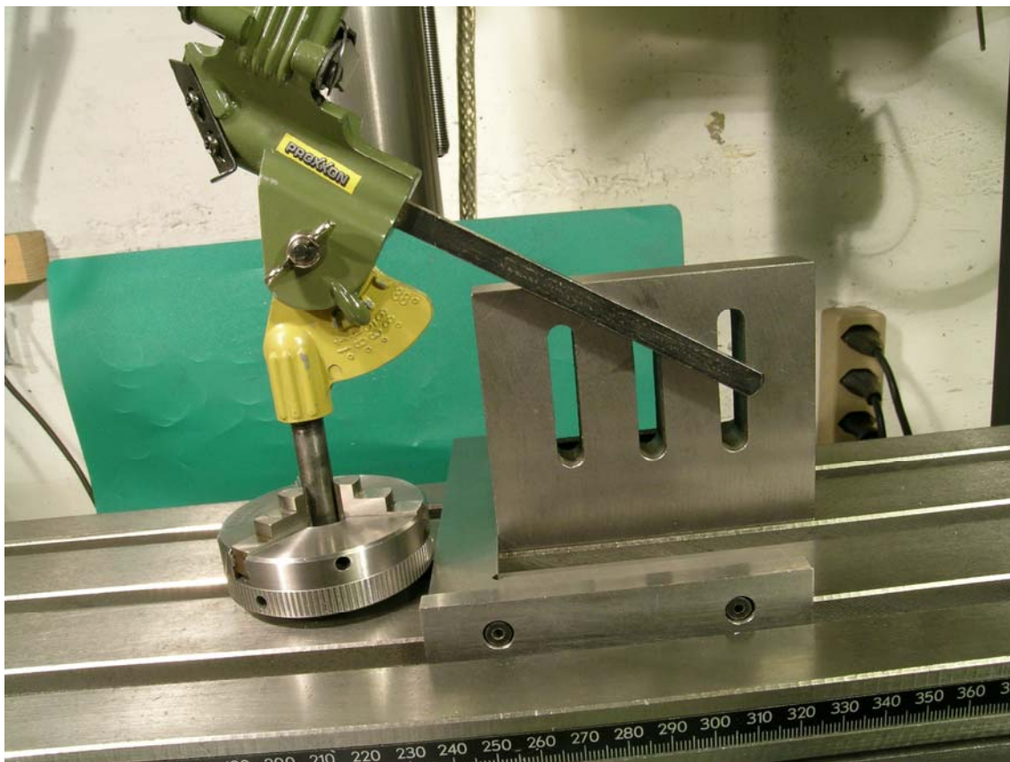
Figure 31: Alignment of the jig to the table's X -axis.
