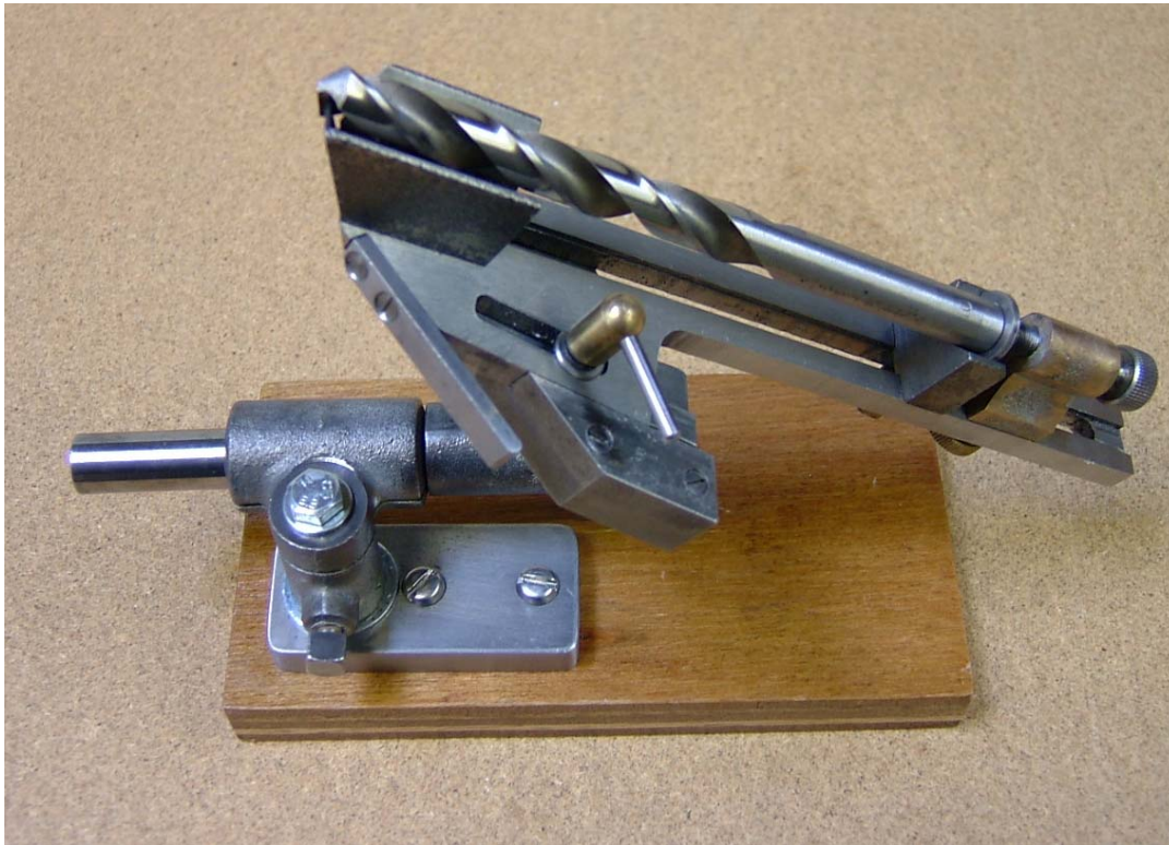
Figure 21: The POTTS drill grinding attachment
